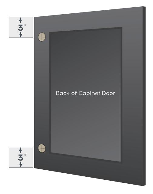
Measure the distance from the bottom & top of the cabinet to the MIDDLE of the bore hole. Standard is 3" offset.
